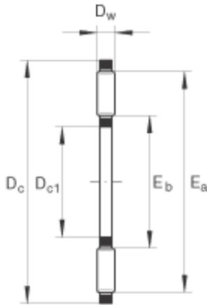
bearing width: INA (Schaeffler) TC2840 Needle Roller Thrust Bearings
